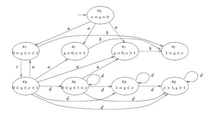
Here transitions that do not change location have been compressed (i.e. each transition in the above graph consists of an arbitrary number of delay transitions succeeded by one action transition)
