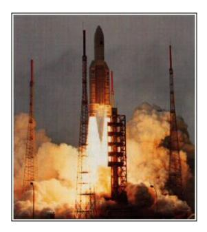
Ariane 5 began to disintegrate 39 seconds after launch because of aerodynamic loads resulting from an angle of attack of more than 20 degrees.
