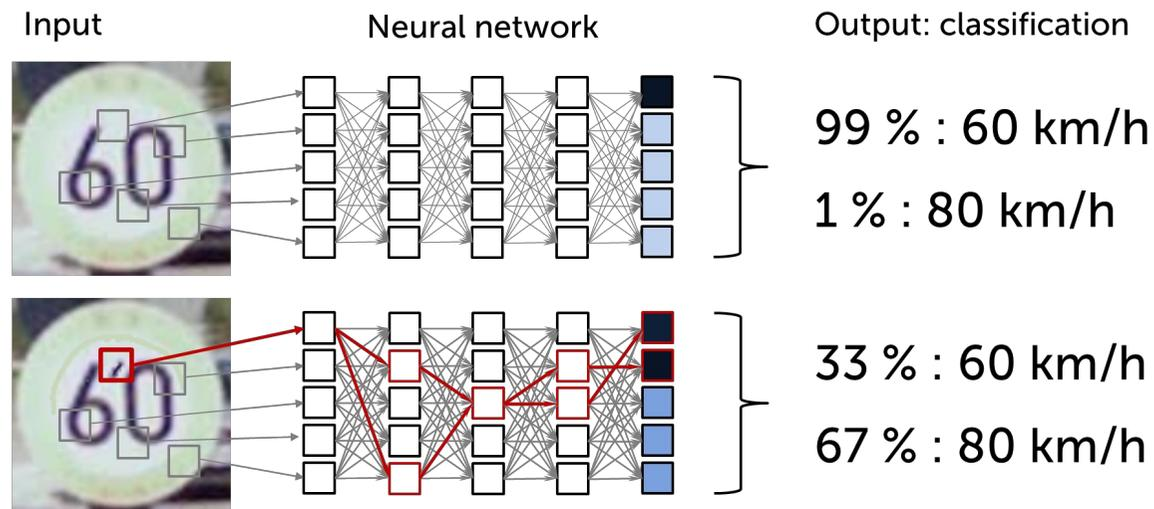
A tiny disturbance in the input causes a significant change in the classification.
