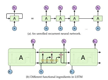
Figure 2.3.: The architecture and details of model RNN and LSTM<sup>1</sup>.
