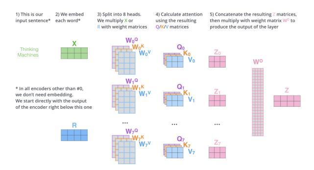
Figure 2.6.: The computational steps of the multi-head self-attention layer<sup>3</sup>.
