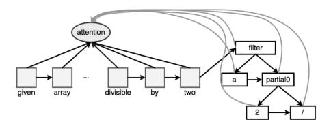
Figure 3.7.: The architecture of Seq2Tree encoder-decorder model.
