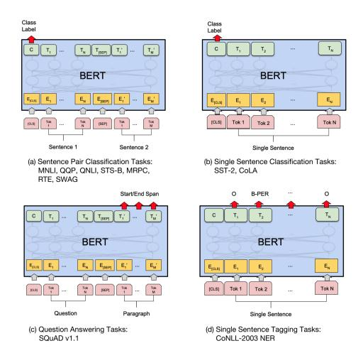
Figure 2.7.: Bert model with one additional output layer for fine-tuning tasks. (a) and (b) are sequence-level tasks, and (c) and (d) are token-level tasks. [24]
