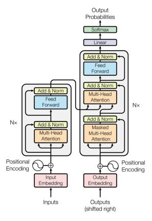
Figure 4.9.: The transformer architecture[21].
