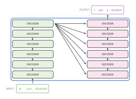
Figure 2.5.: The encoder-decoder transformer architecture<sup>2</sup>.
