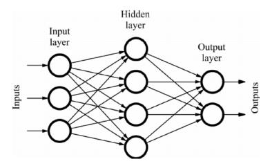
Figure 2.1.: The architecture of a single-layer feed-forward neural network[11].
