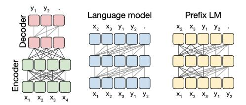
Figure 3.8.: Different transformer architectures. Dark grey lines means the fully-visible masking and light grey lines means the causal masking. The left one is used in the base model.
