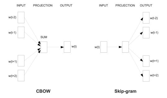
Figure 2.2.: The word2vec models architecture. "The CBOW architecture predicts the current word based on the context, and the Skip-gram predicts surrounding words given the current word.[12]" The weight matrix gives the vector presentation of words.
