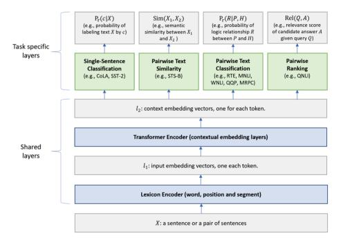
Figure 2.9.: The architecture of Multi-Task Deep Neural Network (MT-DNN) model[32]
