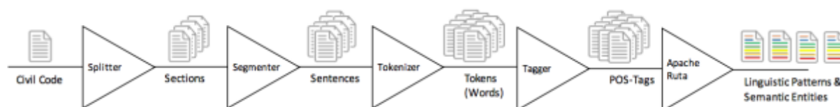
Figure 22: Processing Pipeline for Determining Linguistic Patterns with Apache UIMA and Ruta Source: [168]
