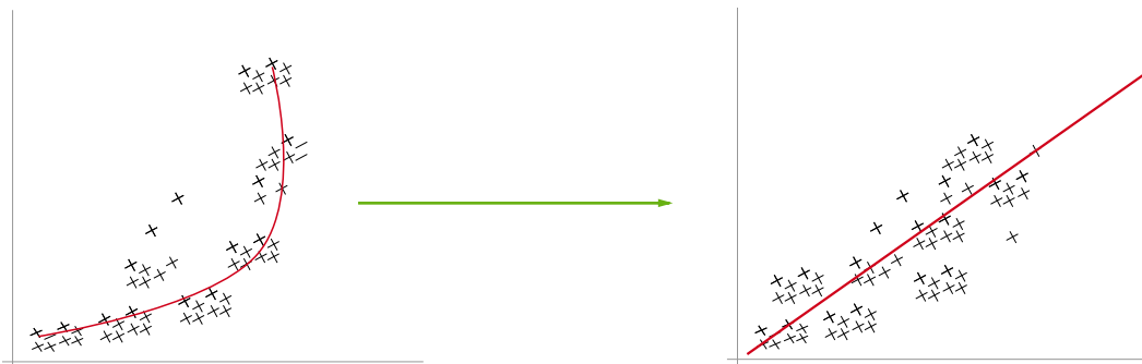
Fig. 6.3: Nonlinear to linear mapping with kernel function
