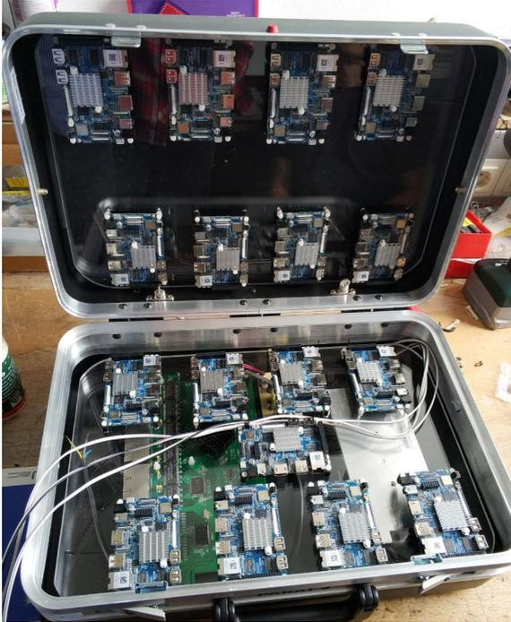
**Figure 3:** The Raspberry Pie Suitcase Cluster: A cluster consisting of Raspberry Pie computers for testing and presenting of the All-Scale architecture.
