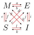
Consider a distributed system with CPUs A, B, C. For a cache line z in the cache of CPU A explain the transition  $b(E \to M), f(M \to S), h(I \to M), i(E \to I)$ , from one state  $s \in \{M, E, S, I\}$  to another state  $s' \in \{M, E, S, I\}$ . Which messages (Read (Response), Invalidate (Acknowledge), Read Invalidate, Writeback (Read Response)) are sent between the CPUs?
