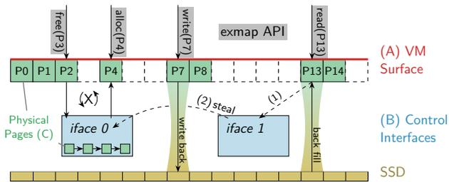
**Figure 5: exmap implementation overview:** The VM Surface (A) is manipulated with explicit free, alloc, read, or write system calls. Each per-thread control interface (B) owns part of the exmap-local memory pool, which exists as interface-local free lists of physical pages (C). If an interface runs out of pages (1), it steals pages from another interface (2). Pages only circulate (X) between the surface and the interface.
