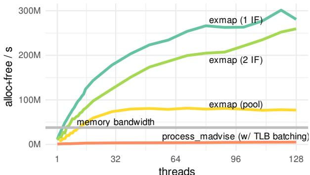
**Figure 8: Linux memory allocation performance with exmap. The three exmap lines shows different page stealing scenarios (1 IF: no stealing, 2 IF: pair-wise stealing, pool: stealing across all threads)**
