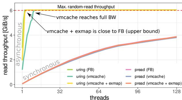
**Figure 9: Read performance for synchronous (pread) and asynchronous (uring) I/O operations. Both vmcache and exmap support asynchronous I/O using uring, which allows achieving full I/O bandwidth using a few threads**
