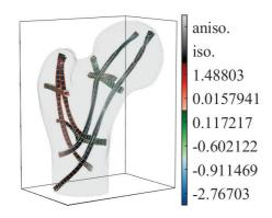
**Figure 16:** *Visualization of stresses in the 3D femur using beams that are grown progressively from user selected seed elements.*
