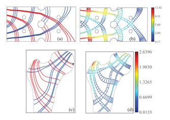
**Figure 11:** Perforated plate (top) and 2D femur slice (bottom). Optimized support trajectories (left), and conforming lattice with von Mises stress encoded along principal directions (right). In the femur stress field, PSLs cannot reach the boundary in the right upper region, because of the two degenerate points (black circles).
