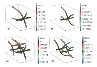
**Figure 15:** Beam structures showing the stresses in the 3D cantilever under different load conditions. Shades of grey characterize the strength of anisotropy of the beam elements. Top: One single seed element is selected. Bottom: Beam structures are extended by growing beams from additional elements.
