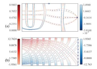
**Figure 10:** *Visualization of stresses in the cantilever under different loads using conforming lattices. Blue arrows indicate the loads corresponding to our 2nd (top) and 3rd (bottom) test case.*
