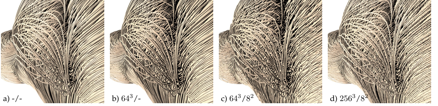
Fig. 5: Rasterization of streamlines in the 256^3 Aneurysm II dataset. (a) Initial lines. (b) Line encoding in 64^3 voxel grid with exact curve-voxel intersections. (c) Line encoding in 64^3 voxel grid with curve-voxel intersections quantized to 8^2 bins. (d) Line encoding in 256^3 voxel grid with curve-voxel intersections quantized to 8^2 bins.
