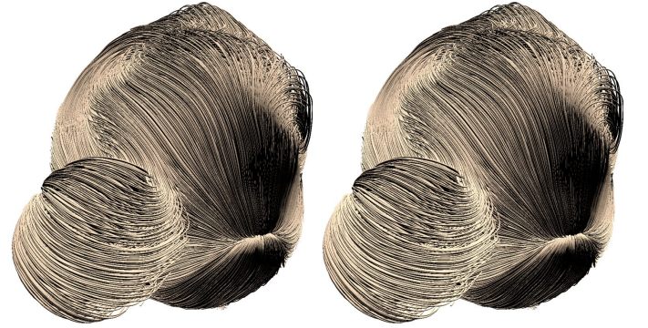
Fig. 10: Opaque line rendering. Left: GPU ray-casting of voxelized lines (8 ms, 256^3 voxel grid, curve-face intersections quantized to 16^2 bins). Right: GPU line rasterization (12 ms).
