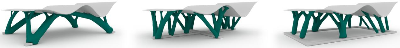
Fig. 16: Variants of optimized roof support structures with different prescribed fixations.
