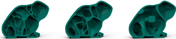
Fig. 10: From left to right: Interior shape variants with increasing minimum thickness. The same external forces are applied, with prescribed volume reduction of 60%.
