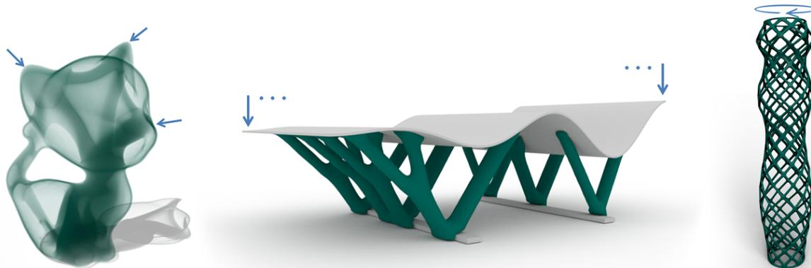
Fig. 1: Shapes generated by optimizing mechanical properties with respect to prescribed loads (blue arrows). The optimization process is applied to interior structures within closed surfaces (left), exposed support structures (middle), and surface models (right). The examples are obtained from an initial solid design domain, targeting a prescribed volume reduction and highest possible stiffness.
