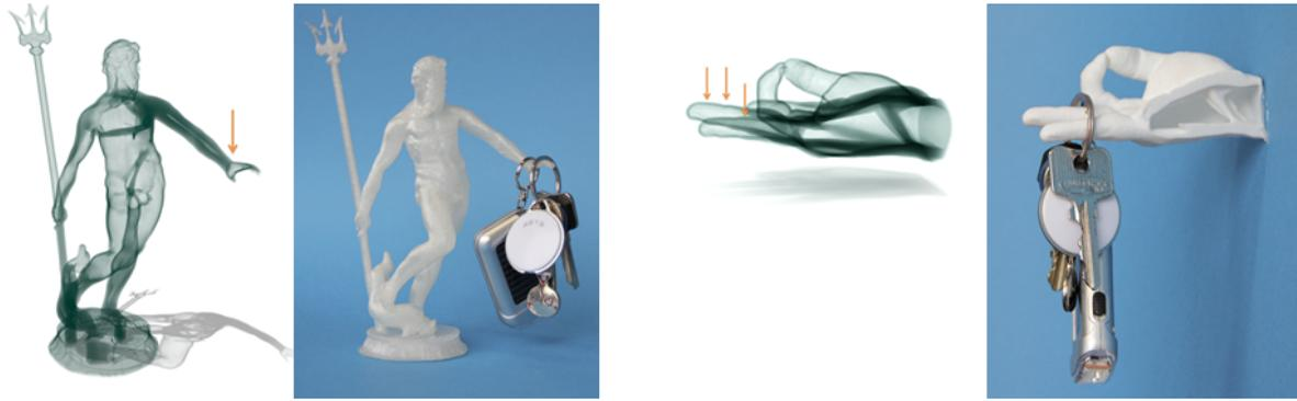
Fig. 12: The Neptune model was discretized on a  $621 \times 488 \times 1000$  grid, with 14.19 million finite elements. Shape optimization took 12 minutes. The hand model was discretized on a  $401 \times 250 \times 178$  grid, with 4.39 million finite elements. Shape optimization took 7 minutes.
