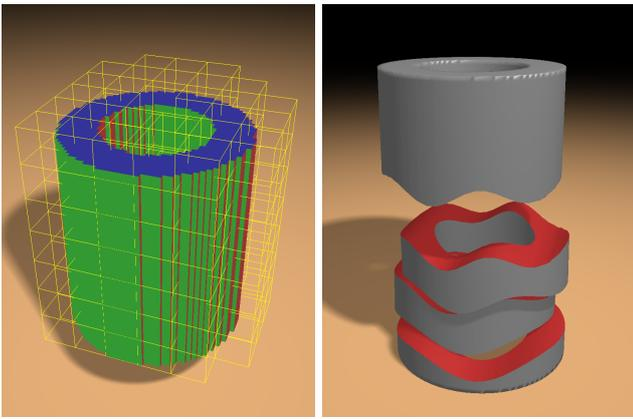
**Fig. 8** Cutting of a cylinder shell model. Left: High resolution hexahedral elements and coarse composite elements. Right: After cutting, the parts fall down and stack. Collision detection and finite element simulation are performed at 136 fps, while the per cut updating is finished in 17 ms.
