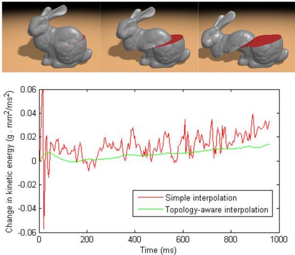
**Fig. 10** Analysis of the change of kinetic energy over time. Top: After cutting the bunny, the upper part slides down. Bottom: With our topology-aware interpolation, the change of kinetic energy (green) is significantly smoother than when the simple interpolation is used (red).
