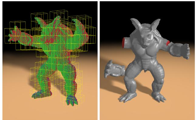
**Fig. 9** Cutting of the Stanford Armadillo model. Left: High resolution hexahedral elements and coarse composite elements. Right: After cutting, the parts fall down. Collision detection and finite element simulation are performed at 30 fps, while the per cut updating is finished in 32 ms.
