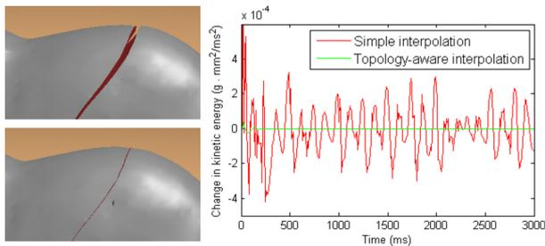
**Fig. 11** Cutting in a zero-gravity environment. Left top: Using the simple interpolation, the cut opens since the collision detection is not accurate. Left bottom: With out topology-aware interpolation, the width of the cut remains zero. Right: Change of kinetic energy over time.
