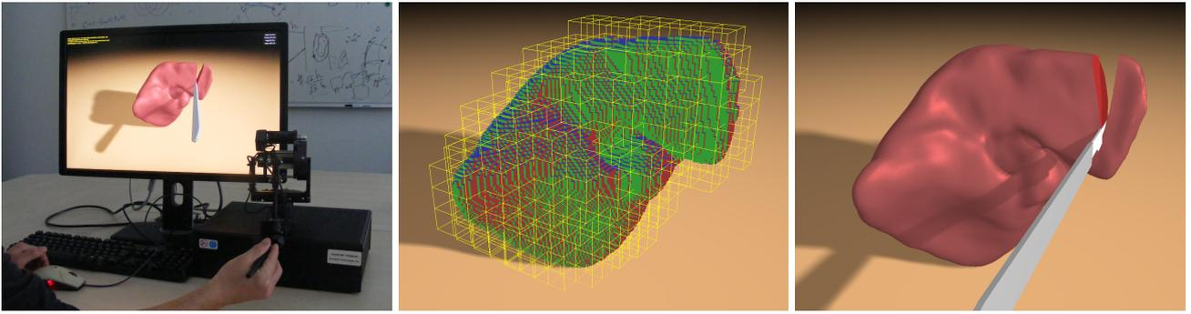
**Fig. 7** Haptic cutting of a liver model. Left: Setup. Middle: High resolution hexahedral elements and coarse composite elements. Right: High quality surface mesh used for visualization. The collision detection between the scalpel and the deformable liver model is performed at 1 kHz haptic rates. Please see the accompanying video for dynamic effects.
