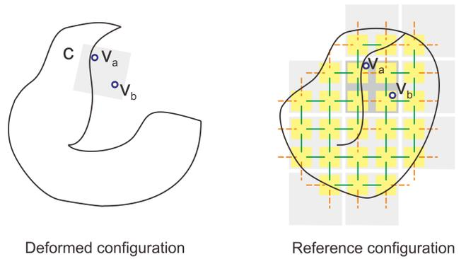
**Fig. 3** Collision detection artifacts at cutting surfaces. In the deformed configuration (left), the vertices  $v_a$  and  $v_b$  are outside the object. Transformed back into the reference configuration (right), the vertices lie inside the object, although in a different material part with respect to the original query.
