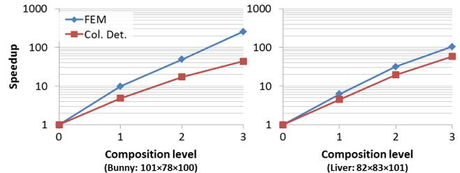
**Fig. 12** Speedup with respect to different composition levels.
