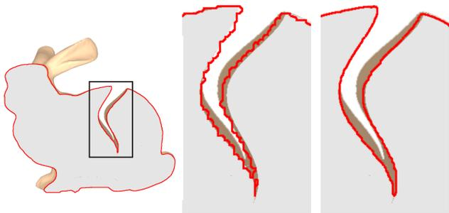
**Fig. 5** Comparison between the zero isocontours of the distance fields obtained by the simple interpolation approach (middle) and our topology-aware interpolation approach (right).
