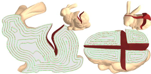
**Fig. 6** Isocontours of the distance field computed directly in the deformed configuration (solid green), and of the distance field computed in the reference configuration and transformed into the deformed configuration (dashed red).
