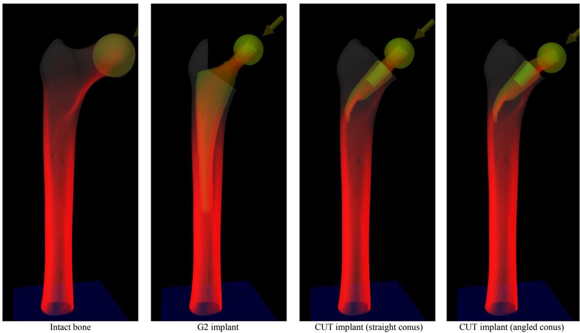
Fig. 4 Visualization of the stress distribution in a femur for the intact bone and three different implants after removal of the femoral head. In all images the same load on the femur was simulated. However, the direction of the force is modified by  $20^\circ$  in comparison with the load in Figure 3.
