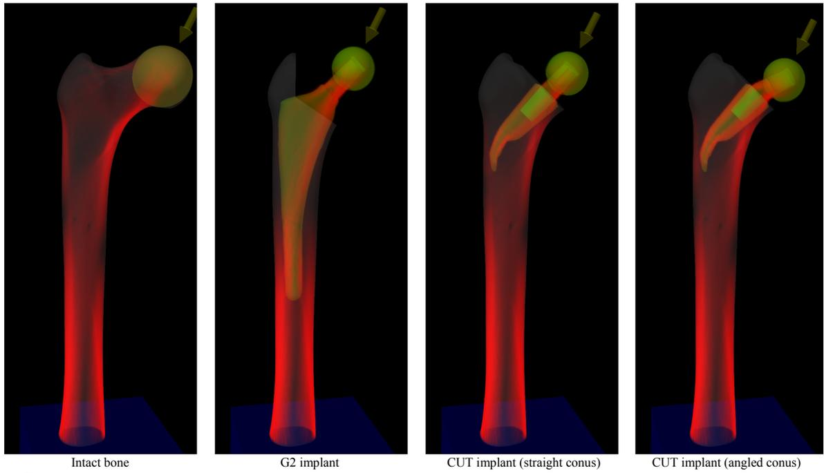
Fig. 3 Visualization of the stress distribution in a femur for the intact bone and three different implants after removal of the femoral head. In all images the same load on the femur is simulated.
