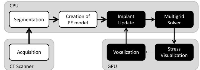
Fig. 2 Overview of the main components of the implant planning system.
