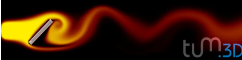
Fig. 2. Simulation of the Karman Vortex Street on a 256x64 Grid is shown. The simulation and rendering runs at 400 fps using our GPU framework on current ATI hardware
